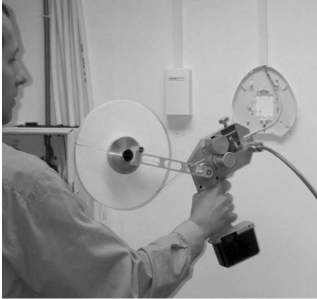
Figure 3.12 Ericsson delivers a wide range of broadband access products. Here is an example of a handheld, battery-powered fibre-blowing tool used in the Ribbonet ® solution. (Courtesy of Ericsson). Reproduced by permission of Ericsson.
