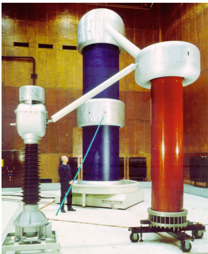
Fig. 2.6 Two-stage 800 kV transformer cascade housed in insulating cylinders (in the background) with compressed-gas capacitor (right) and instrument transformer (left) in the foreground (PTB)
