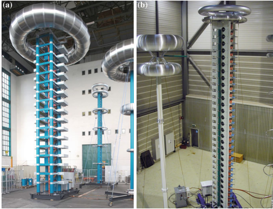
Fig. 4.12 Two types of impulse voltage generators. a Total charging voltage 3.2 MV, 320 kJ (HIGHVOLT Prüftechnik Dresden GmbH). b Total charging voltage 3 MV, 300 kJ (Haefely Test AG)
