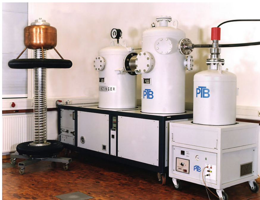
Fig. 3.6 SF 6 -insulated 300 kV DC voltage supply (left-hand metal tank, background) connected with a 300 kV voltage divider (large metal tank in the middle), a separate SF 6 -insulated 100 kV voltage divider of the highest accuracy (right) and an older oil-insulated 300 kV voltage divider (left) (PTB)
